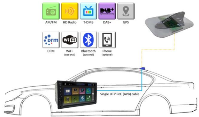
Multimedia Gateway with active antenna and various RF functions
