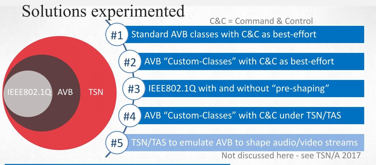
Several mechanisms to ensure QoS w.r.t. timing , but which are the most efficient for automotive systems?
