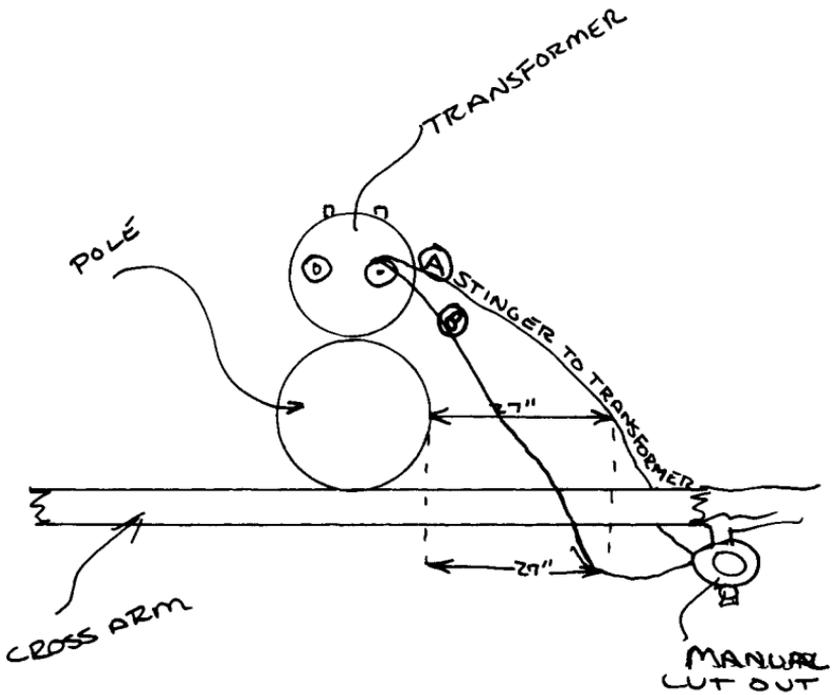
Fig IR 176-3. (1) Does climbing space extend into this stinger wire if mounted in the position of stinger A? (2) Does climbing space extend into this stinger wire if mounted in the position of stinger B?
