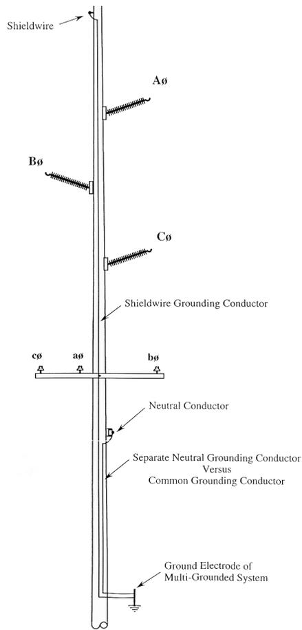
**Figure 1—Typical wood transmission structure with distribution underbuild**
