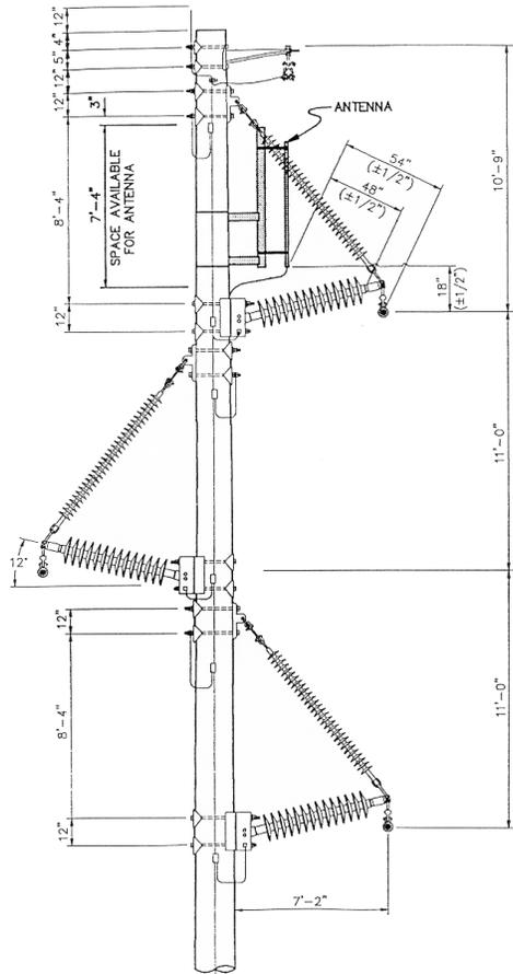
**Figure 2—PCS antenna, pole top assembly**
