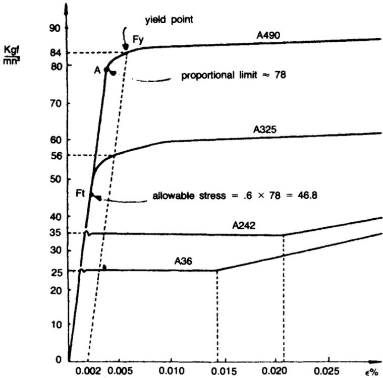
Stress-strain diagram of selected ASTM structural steels
