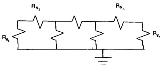
The total neutral-to-earth resistance looking across  $R_{G_4}$  is .68 ohms.
