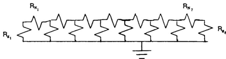
The total neutral-to-earth resistance looking across  $R_{g_8}$  is 1.11 ohms.
