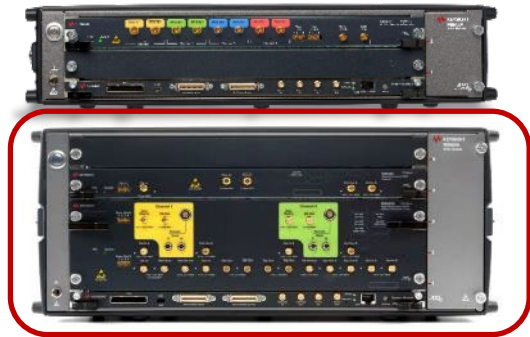
Bit Error Ratio Tester (BERT) with Pattern Generator (PG) Optical Reference Transmitter for stressed signal generation Oscilloscope to calibrate stressed eye signal
