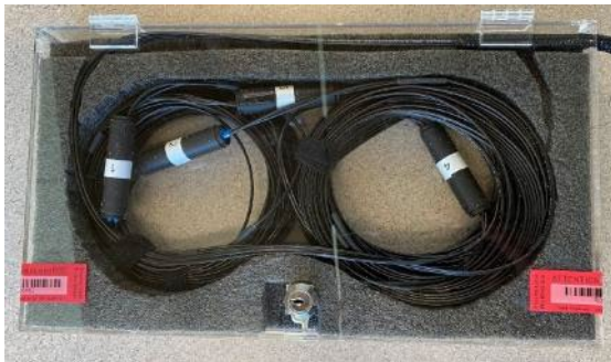
40m glass optical cable with 4 inline connectors
