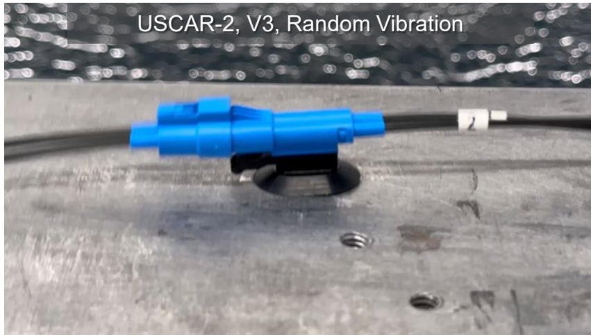
Connector in vibration (random) testing
