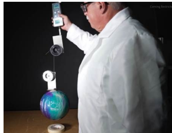
~11lb Bowling ball hanging from 125um multimode glass optical fiber
