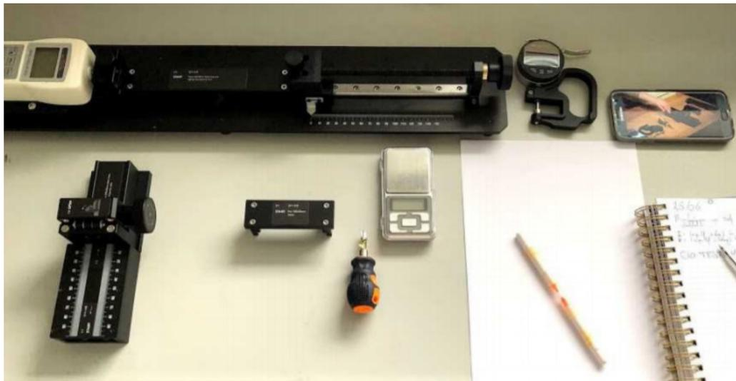
In total, one warp, one weft, and one bias fabric specimen, each of 22 cm by 3 cm, are required to measure the weight, thickness, bending, and tensile properties.
