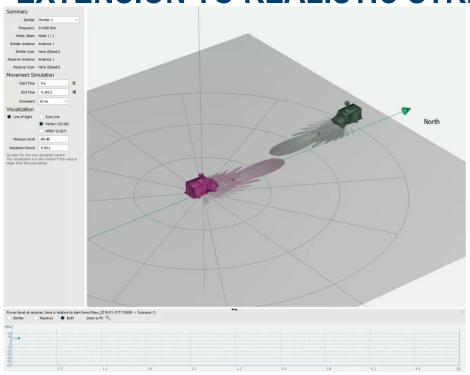
The R&S®Pulse Sequencer can generate realistic scenarios, including but not limited to following parameters:
